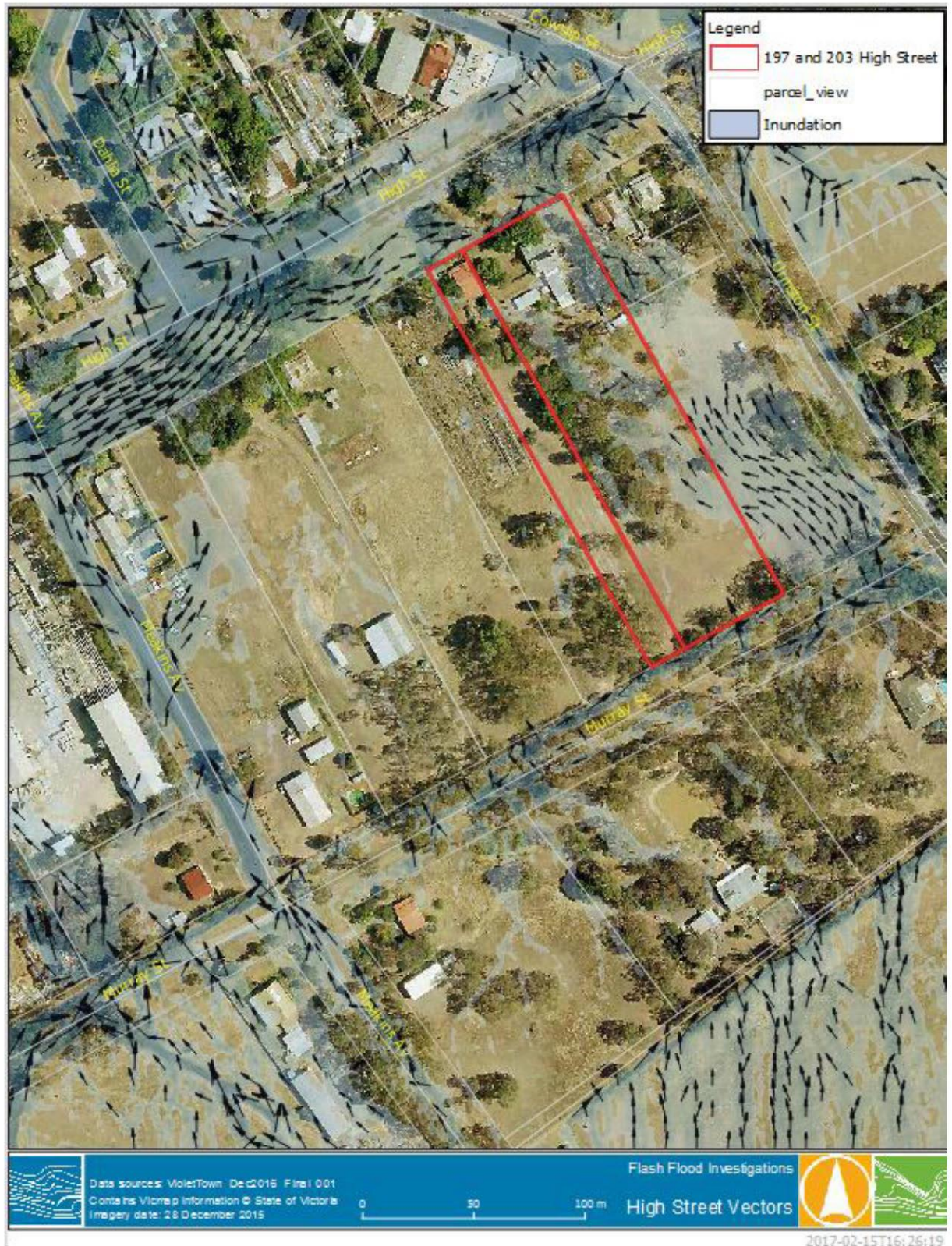
Figure 3-2 Overland flow paths impacting properties on High Street, Violet Town
