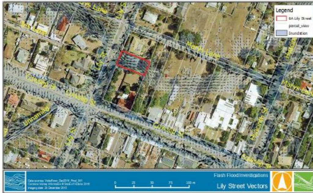
Figure 3-3 Overland flow paths impacting 6A Lily Street, Violet Town
