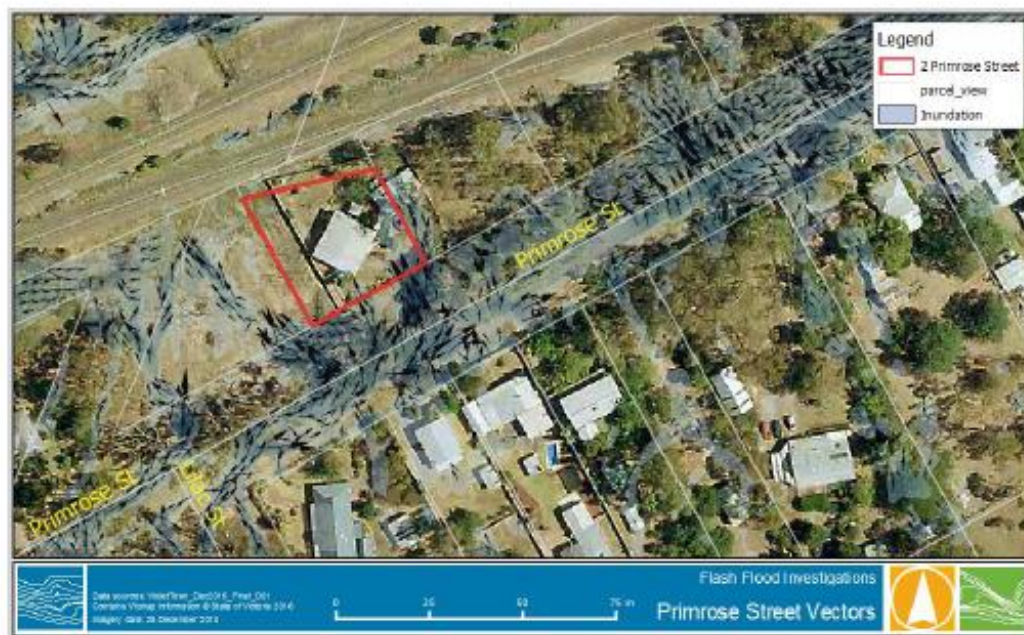
Figure 3-4 Overland flow paths impacting 2 Primrose Street, Violet Town
