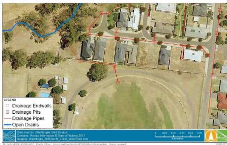
Figure 2-3 Drainage network at the Nagambie site
